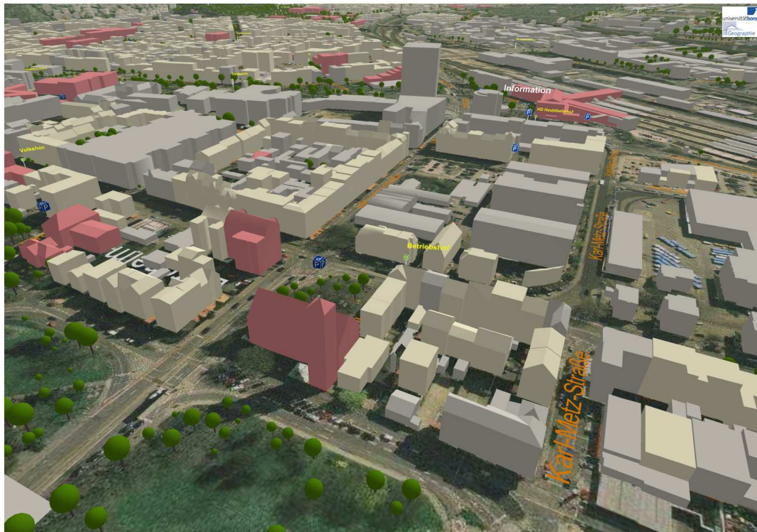
Fig. 2: User-defined Styling. The buildings are colored according to the usage type (public, mixed, private). Trees are portrayed as prototypic inline objects whose size is controlled by an attribute.
